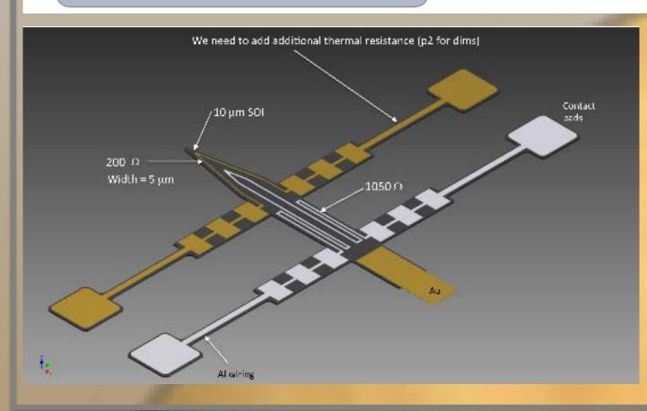
Isolation is also important to avoid contaminating the received signal with the calibration power, and need to be 25 dB or greater. Shown is the switch module design (top), and the temperature controlled load. The load will allow multitemperature calibration.
