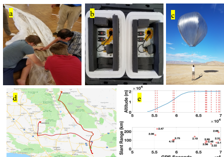
Figure 3. (a) Fabricating the 6-meter balloon envelope; (b) Ready the instrument box for launch; (c) Balloon launch on July 22; (d) Flight trajectories on July 22; (e) Balloon altitude and intercepted aftershocks events.
