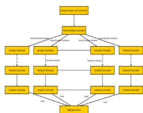
Figure 2. The search algorithm is based on a Monte Carlo simulation of execution where multiple schedules are generated during each execution simulation.
