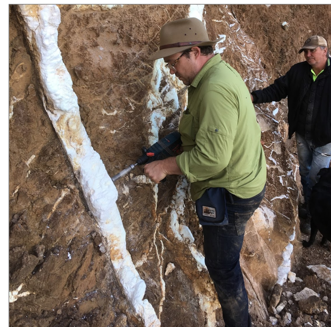
PI Williford acquires a sample of Jezero-analog Kunwarara magnesite (QLD, Australia) using a Mars 2020 drill bit.
