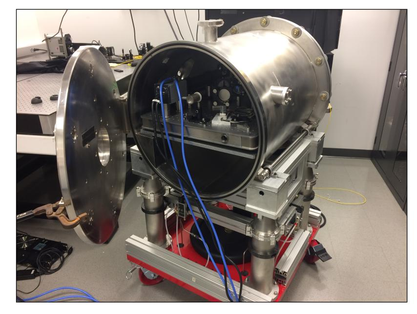
The VERVE Instrument is a single-mode fiber-fed externally dispersed echelle spectrograph. It covers the visible portion of the spectrum with a resolving power of ~ 20,000.
