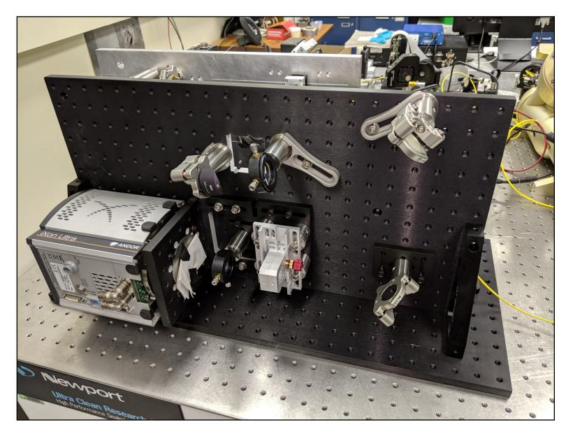
The final, fully assembled hardware is shown in this figure. The plate closest in the image shows the pyramid wavefront sensor. The hidden vertical plate has the optical relay with the deformable mirror and fiber injection optics.
