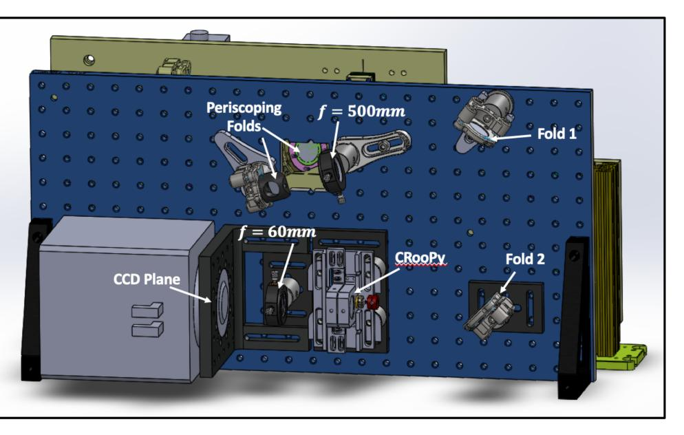
The wavefront sensor arm of the Compact AO system used a transmissive pyramid wavefront sensor. This wavefront sensor arm enhanced the nominal DM relay design from the Keck Planet Imager and Characterizer (KPIC).
