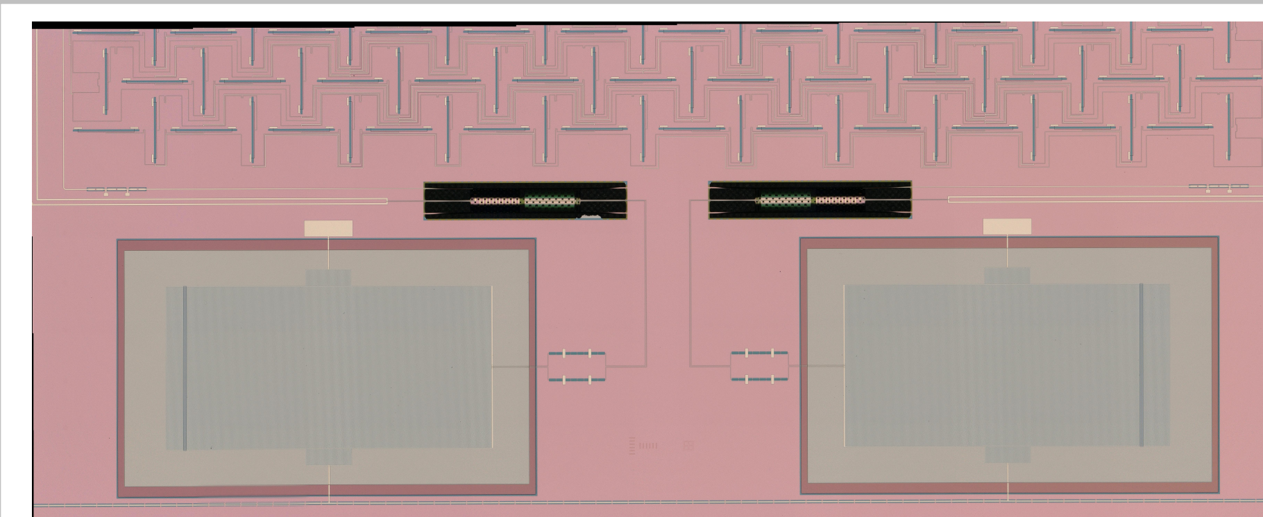
Figure 1: Microscope images of antenna coupled TKIDs. Results on this poster are from detectors without the antenna, but otherwise identical. Antenna coupled measurements currently underway.
