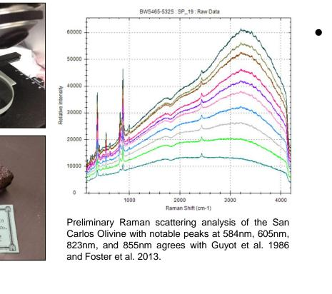
To represent the chondritic interiors of ocean worlds, we use samples of olivine, fayalite, and added Fe/Ni to represent various reactive chondrite materials. Electrodes are made by painting these samples onto an electrode and incorporated into the test bed reactor.
