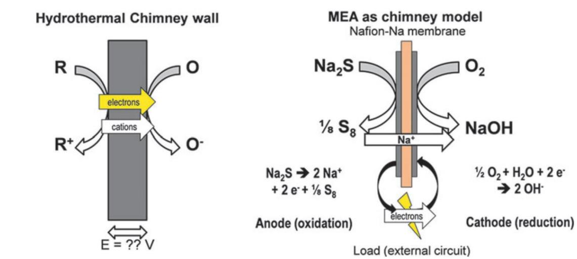
The mineral-driven redox reactions of a hydrothermal vent can be modeled as a fuel cell: the cathode and anode contain conductive / catalytic minerals, driving abiotic or biotic redox reactions that that are electrically linked, affecting potential metabolisms in these systems. (Barge et al. 2018, Astrobiology, DOI: 10.1089/ast.2017.1707)
