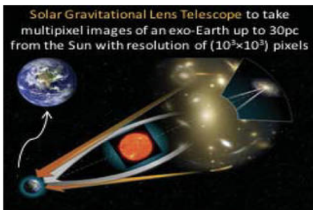
Figure 1. Interstellar precursor mission to 500 AU to use the sun as a Gravitational Lens. Requires Li ion thruster to get there in <12 yrs.
