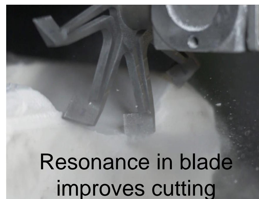
Powder-bed 3D printing of tools
