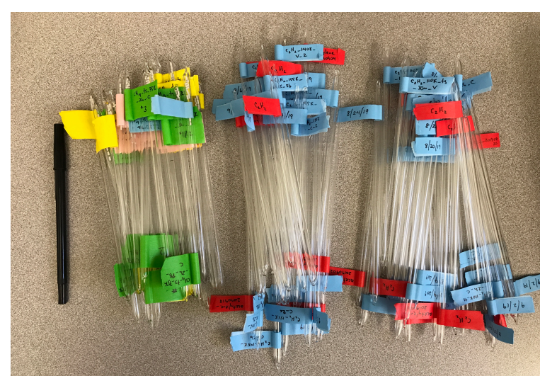
Figure 2. 'Breakseals': Pyrex tubes into which experimental reactants and products are frozen for storage prior to analysis. Tubes are cracked in an evacuated, custom-designed Swagelok apparatus and gases are extracted using gas-tight syringes for injection into the GC-pyrolysis isotope ratio mass spectrometer for isotopic analysis. Experiments presented at left are awaiting analysis. Pen for scale.
