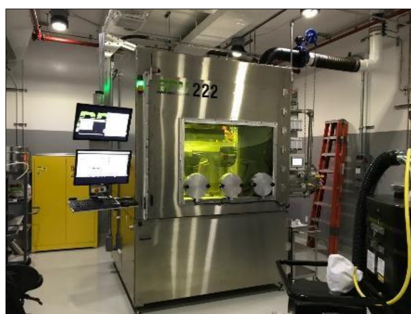
JPL's RPM 222 Directed Energy Deposition (DED) System
