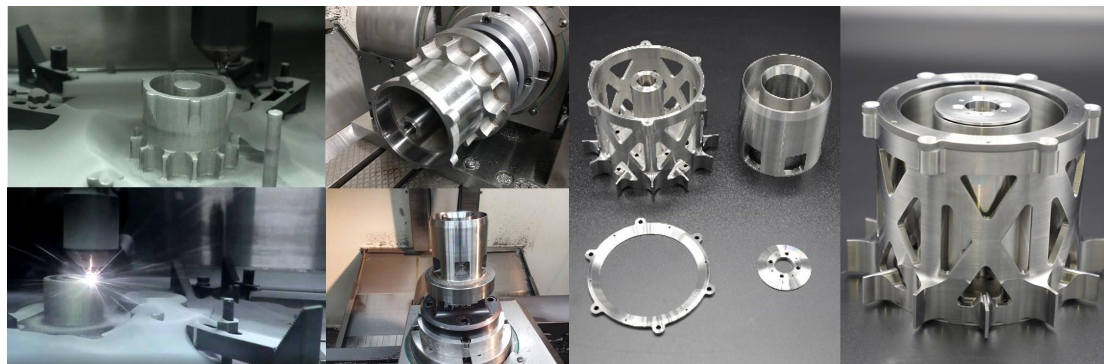
Manufacturing models of the core, screen, and pole pieces were printed, machined, and heat-treated. Initial testing indicates the magnetic performance is in-family with a traditionally manufactured (fully machined) thruster of the same design.
