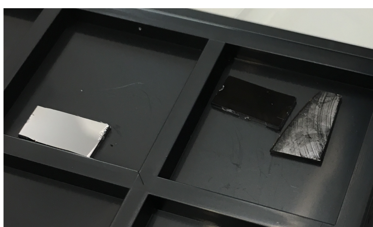
Fig. 4: Three single-pixel HOTBIRD devices, upside-down. Left to right: untreated, polished-then-etched, etched without polishing.
