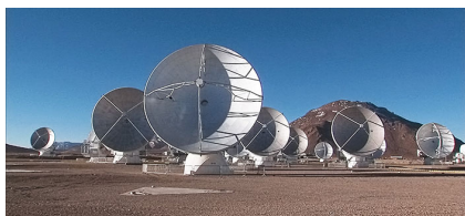
The Atacama Large Millimeter Array used for long-baseline heterodyne imaging of celestial objects.
