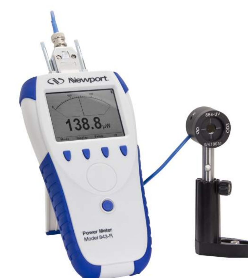
818-UV/DB low power UV enhanced silicon photodetector with an 843-R optical power meter (Newport, Irvine, Ca)
