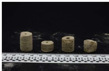
3D printed olivine sand coupons
