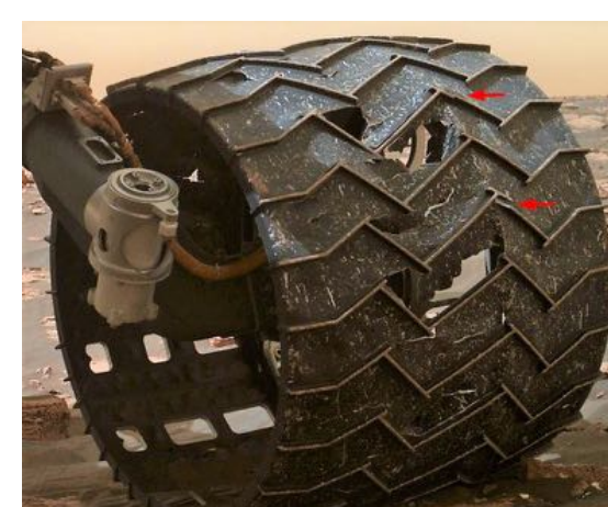
Wheels of Curiosity rover got damaged
