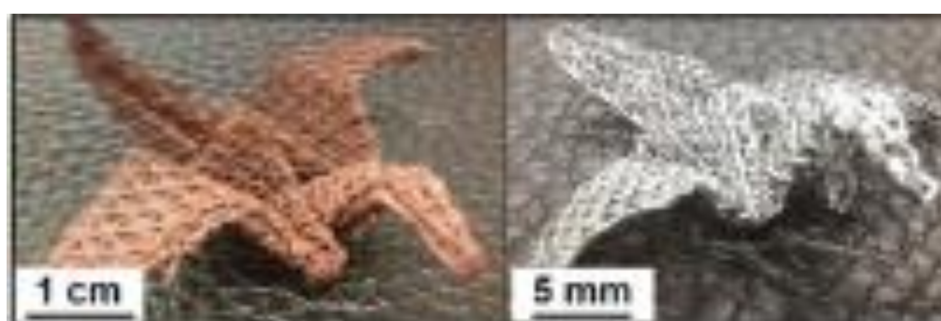
Conversion of printed \text{Fe}_2\text{O}_3 structure in to metallic \text{Fe} . 3
