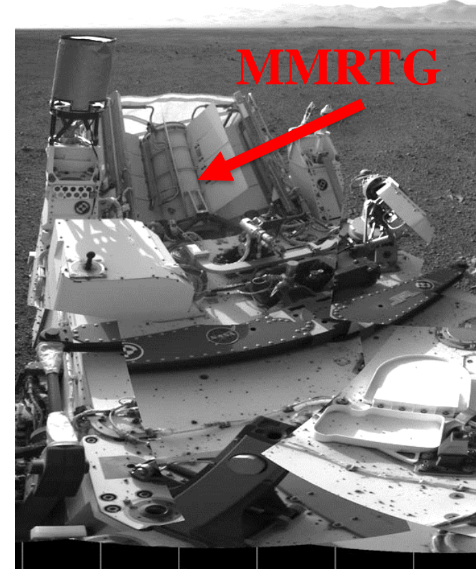
(Left) Radioisotope heat source used in RTGs. (Right) Image of Curiosity 's Multi-Mission Radioisotope Thermoelectric Generator (MMRTG). 1
