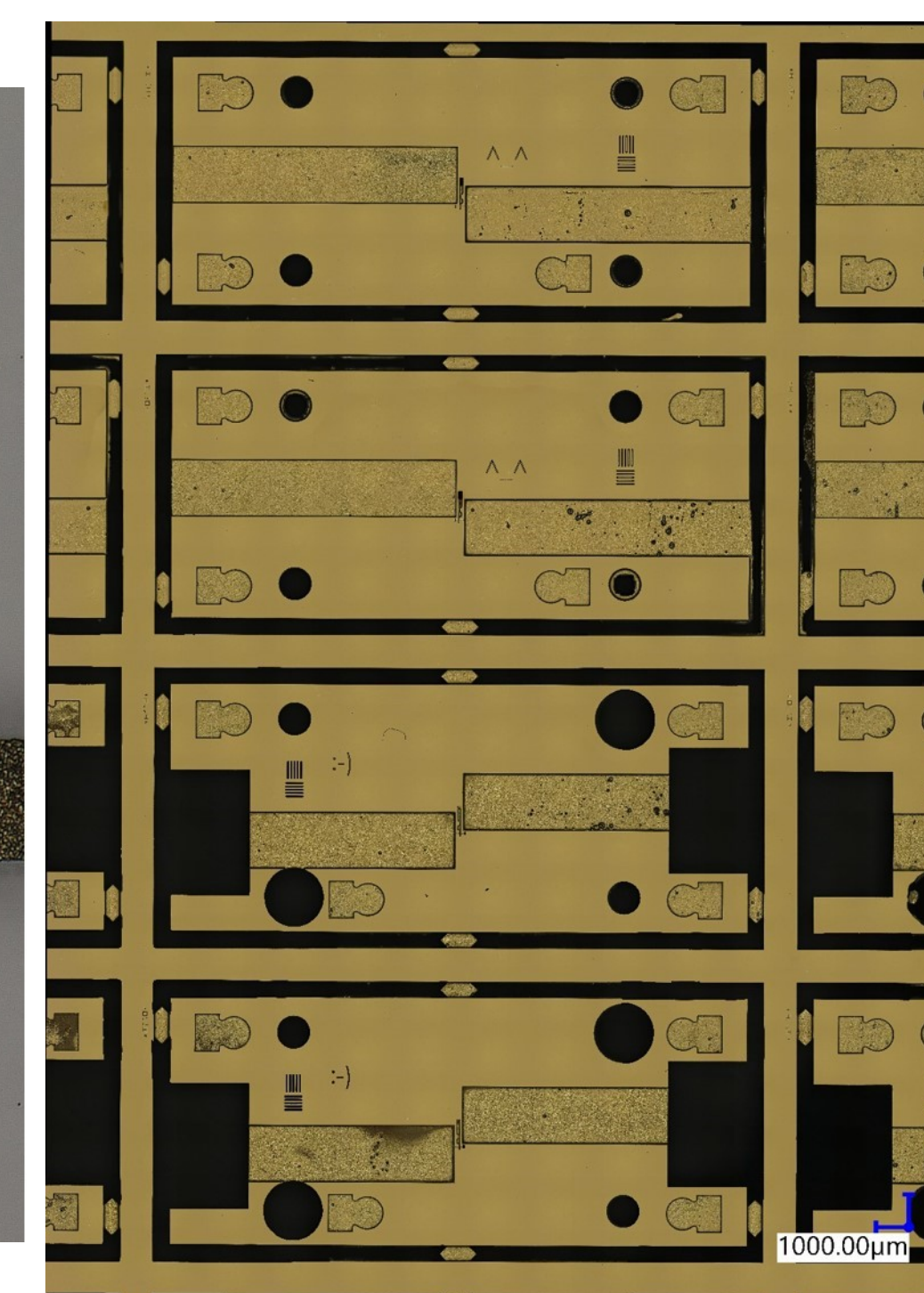
[Figure 3: Top-down microscope image of top and bottom stack on 4" Si wafer]
