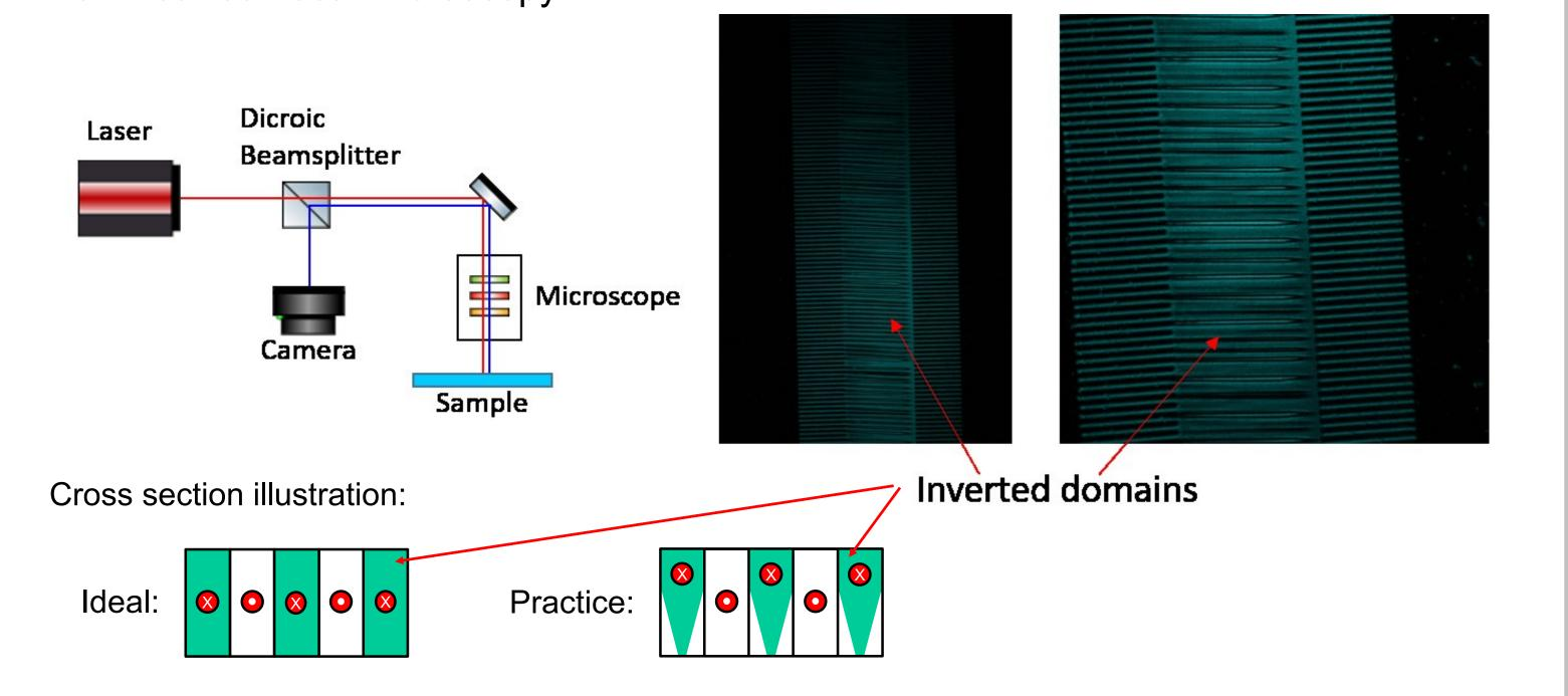
The objective of this R&TD task was to develop a process for the reversal of ferroelectric polarization domains within a thin-film lithium niobate crystal.
