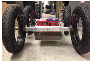
End-view and ground clearance of GPR antenna on Dasher prototype
