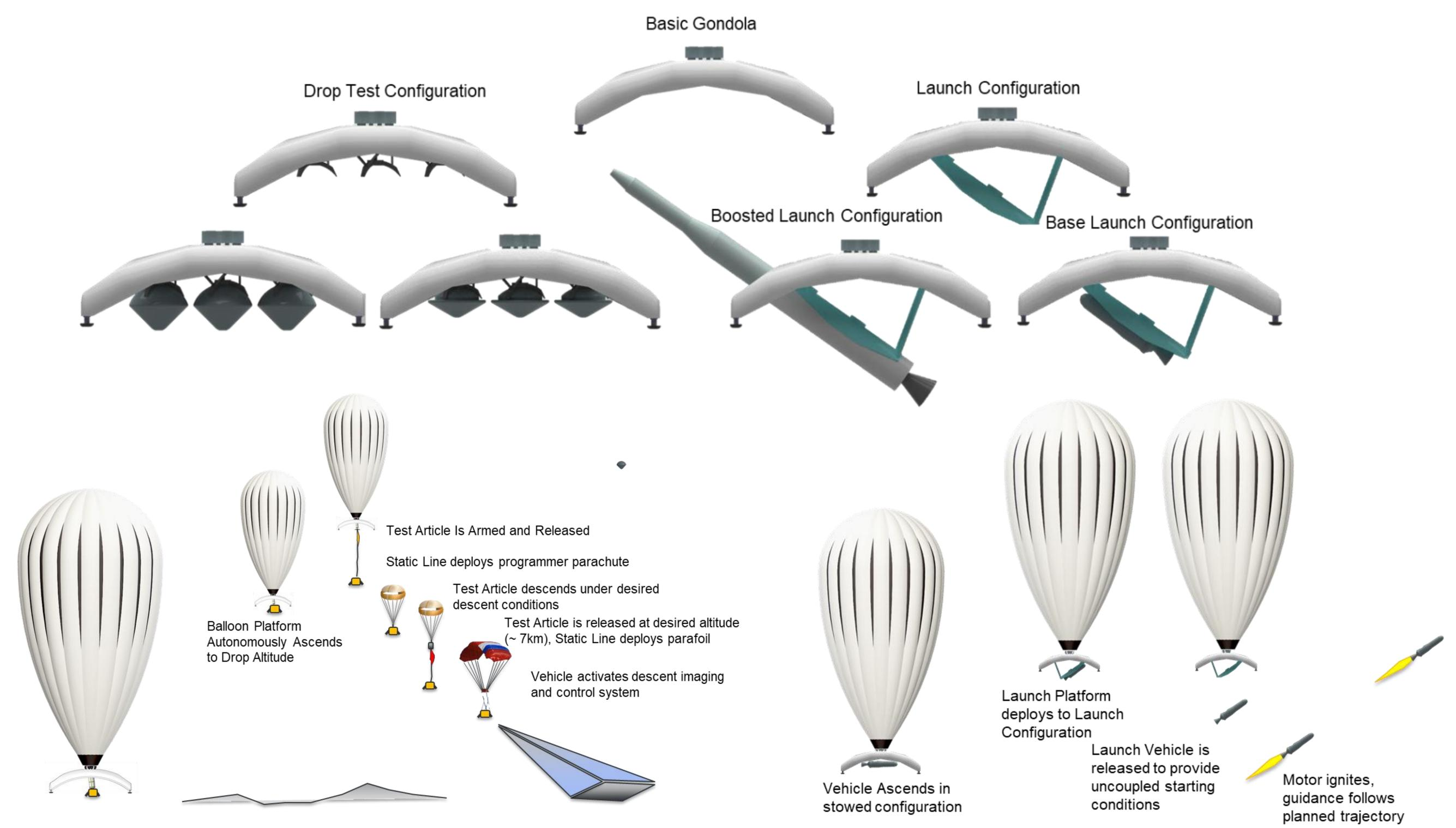
Titan Parafoil Drop test concept for verifying performance at 30-40 km altitude equivalent conditions
