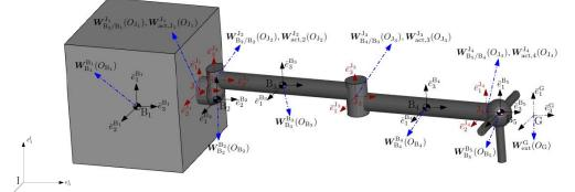
Geometry of a spacecraft-manipulator system with centers of mass, coordinate frames and wrench definitions
