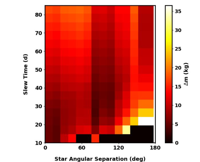
$\Delta m$  fuel costs for continuous thrust maneuvers. Results only shown for a subset of angular separation, this is an intermediate product. Still shows continuity exploitable through a 2-D interpolant as before.
