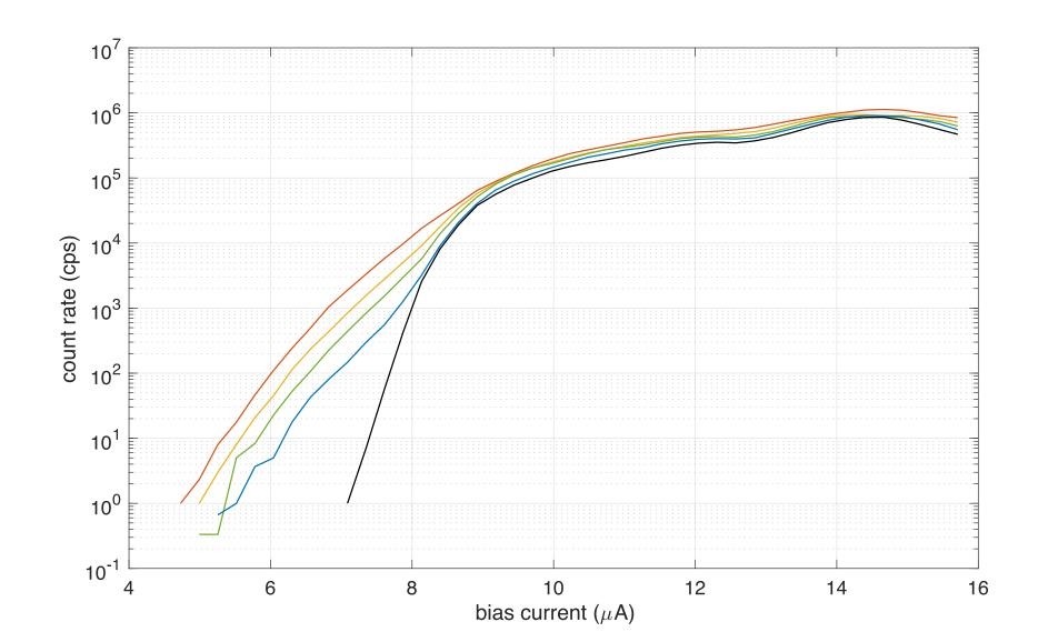
Count rate vs. SNSPD bias for different applied optical powers measured with optical readout. The detector is photosensitive in the regime where changing power results in changing count rate. The detector undergoes power-independent relaxation oscillations
