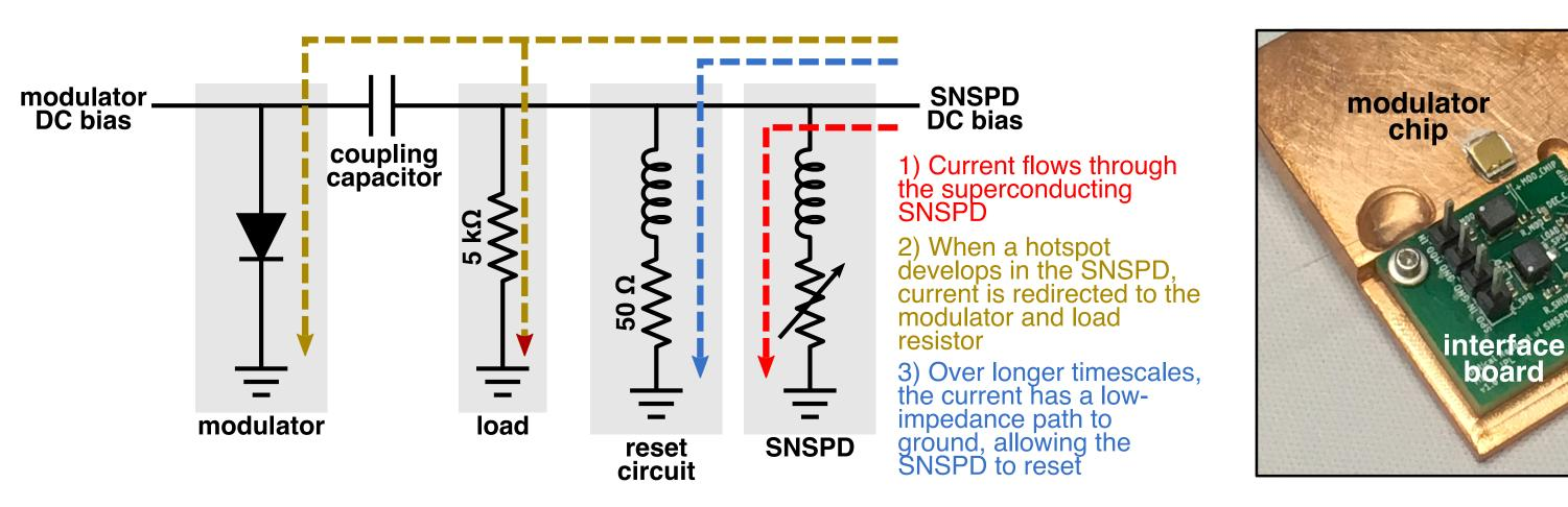
Simplified circuit schematic showing the operational principle of the demonstrated readout scheme. For a proof-of-principle demonstration of optical readout, we combined existing modulator and SNSPD chips using an interface PCB. All components were operated at 3.6 K.
