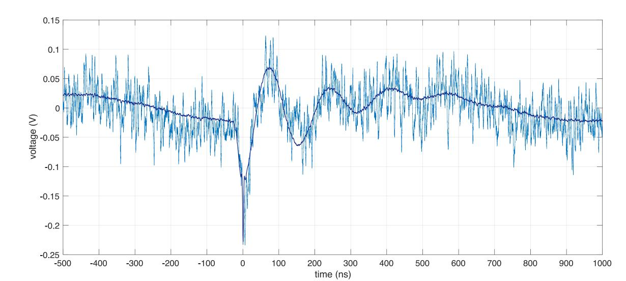
First demonstration of optical readout of an SNSPD: voltage signal from a photodiode showing the SNSPD's modulation of the optical carrier. Signal-to-noise was limited by optical losses.
