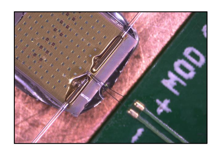
Optical micrograph of the modulator chip showing the input and output optical fibers. Attaching the fibers to the chip in such a way that they would stay aligned with the on-chip grating couplers at low temperatures was a challenge. The total optical losses in our final device were 30 dB, but it is expected that this can be improved to 6 dB.
