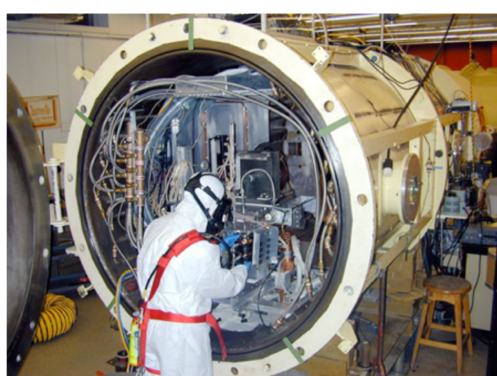
Fig. 8: Princeton's lithium test chamber—specifically designed to test high power lithium-fed engines. The feed system was modified to deliver the low flow rates required for the ion source.
