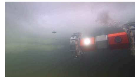
A prototype of NASA's Jet Propulsion Laboratory's Buoyant Rover for Under-Ice Exploration, a technology that could one day explore oceans under the ice layers of planetary bodies, being tested in a lake near Utqiagvik, Alaska.
