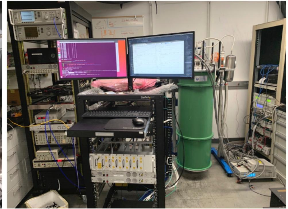
Readout uses ROACH-2 electronics with firmware developed by ASU and software developed by KID consortium including Caltech, NIST, Chicago/Argonne
