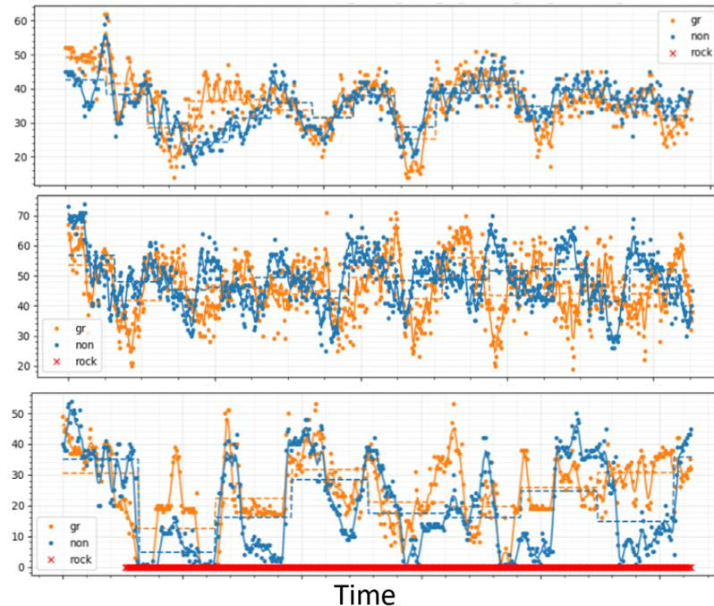
Contact area time series for **low slip/flat**, **high slip**, **rock** (top to bottom) contact area with wavelet and mean filter smoothing. Each type of experiment has a unique signature.
