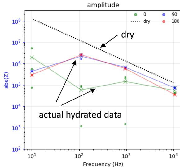
In-motion EIS experiment with **10%** hydration shows distinct moisture signature, however, data appears to be very noisy in general and requires good contact with the ground.
