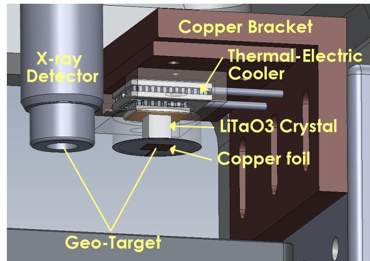
**Figure 1:** Single crystal and copper film schematic of 1-crystal pyroelectric instrument design planned for development in the forthcoming year. Instrument testbed key components include 1-crystal source and Amptek XR-100SDD detector and Amptek PX5 Digital Pulse Processor.
