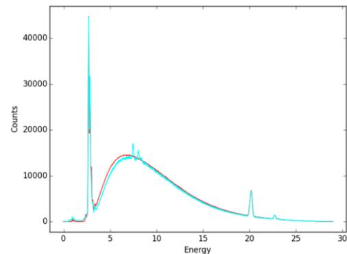
Figure 6: pyPenelope MC calculation for PIXL flight measurement of Teflon compared to PIXL Teflon data.
