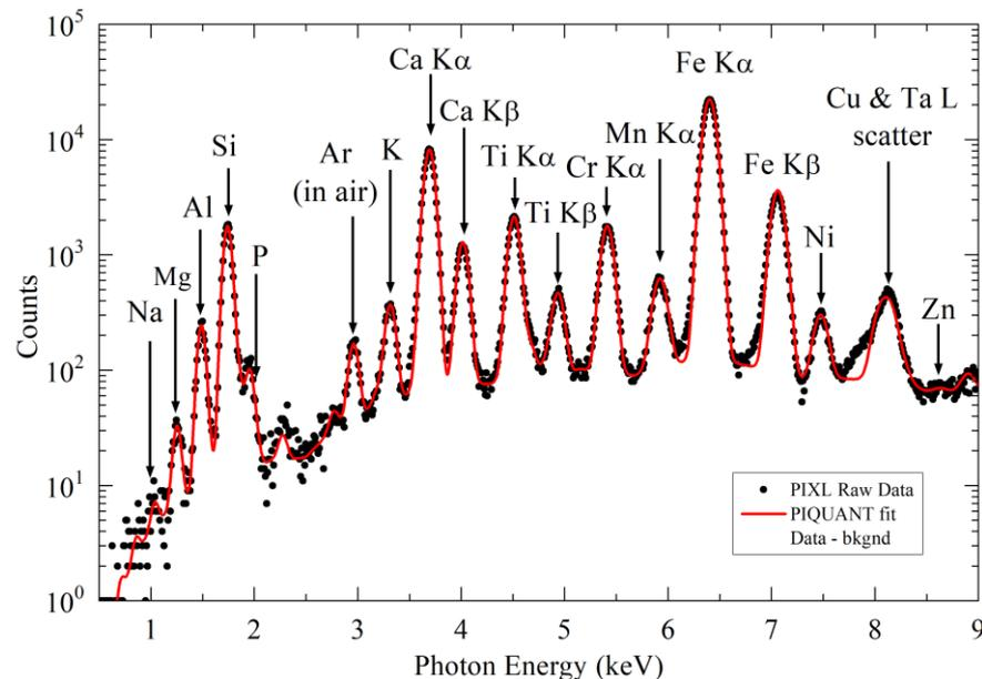
Figure 7: Histogram of geological reference material BHVO2 powder measured using Amptek Cool-X in helium environment for 75 minute equivalent single detector integration. Major and minor elements in sample identified in 0 – 9 keV range.
