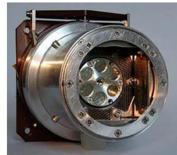
Figure 2: Mars Science Laboratory Alpha-Particle X-ray Spectrometer (APXS). Source: <https://mars.nasa.gov/msl/spacecraft/instruments/apxs/>
