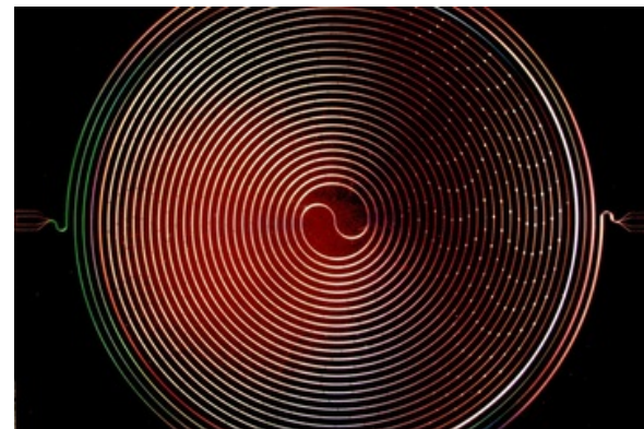
An NbTiN kinetic inductance parametric amplifier based on a spiraled thin film transmission line.
