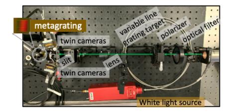
Config. #1: delivers spatially, spectrally, polarimetrically, resolved images Config. #2: the measured polarization contrast, polarimetric modulation, and spectral resolution agree to the theoretical prediction
