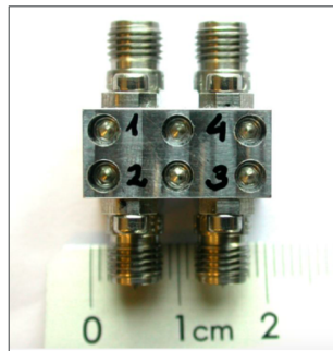
Yebses Observatory 8-40 GHz Cryogenic Quadrature Hybrid.
