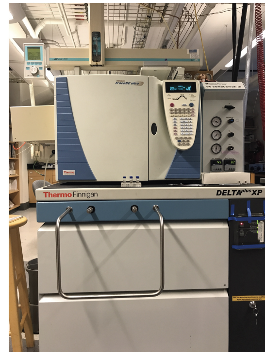
Figure 4. The mass spectrometer with dedicated gas chromatograph at Caltech used to analyze experimental products and starting materials in this study .
