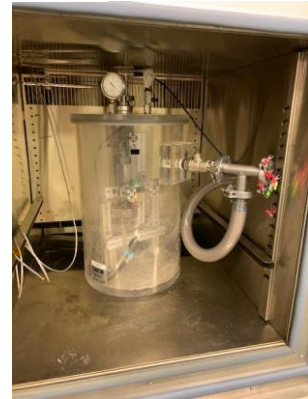
Tvac system for in-situ geochemical measurements under Lunar or Mars conditions.
