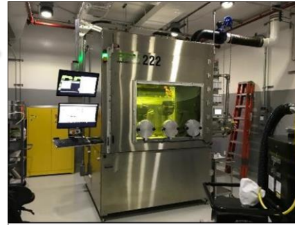
JPL's RPM 222 Directed Energy Deposition (DED) System
