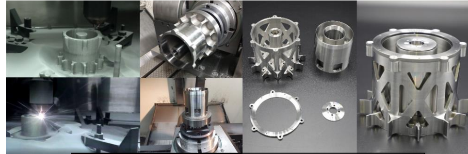
MaSMi core and screen components and manufacturing models used for printing
