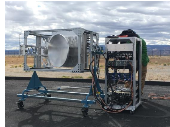
JPL's VIPR radar system, developed under IIP-16, is the foundation of the orbital differential absorption radar concept. It measures humidity profiles inside of clouds, and total water vapor columns, with accuracy better than 1 g/m 3 .
