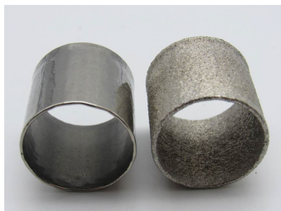
Established process for chemical surface finish enhancement after printing (vendor)
