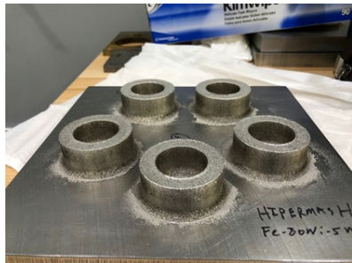
Measured magnetic properties of printed test coupons with a variety of post print thermal treatments
