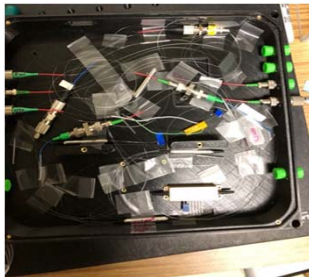
JPL built the Fiber Laser Comb which will be used to stabilize the microresonator
