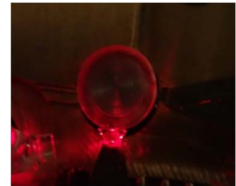
The WGM resonator etalon light coupling at OEwaves (left), etalon spectrum pumped at 1550 nm showing 10 GHz line spacing (center) and with 633 nm light at JPL (right).
