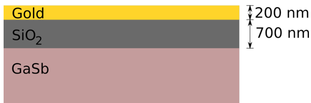
Cross-section view of the filter structure.
