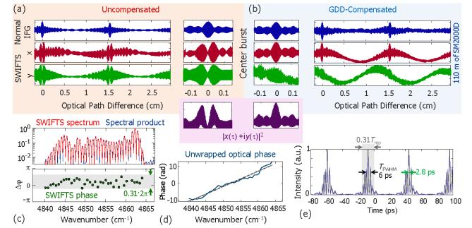
Around ZPD, the rf beat note IFG has a sharp peak indicating strong amplitude modulation.
