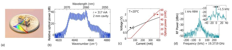
Combs demonstrate broad optical spectrum (> 20nm) with low intermode beat node phase noise
