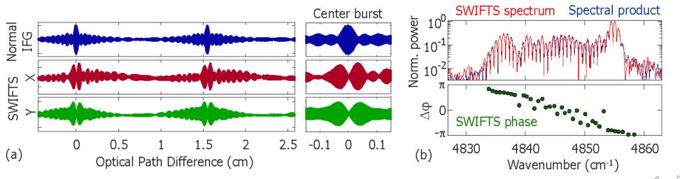
A characteristic minimum around the zero-path-difference (ZPD) point visible in the SWIFTs traces confirms the FM character. Additionally, the phase difference between neighboring lines varies almost linearly from  $\pi$  to -  $\pi$  as expected for a maximally chirped comb state
