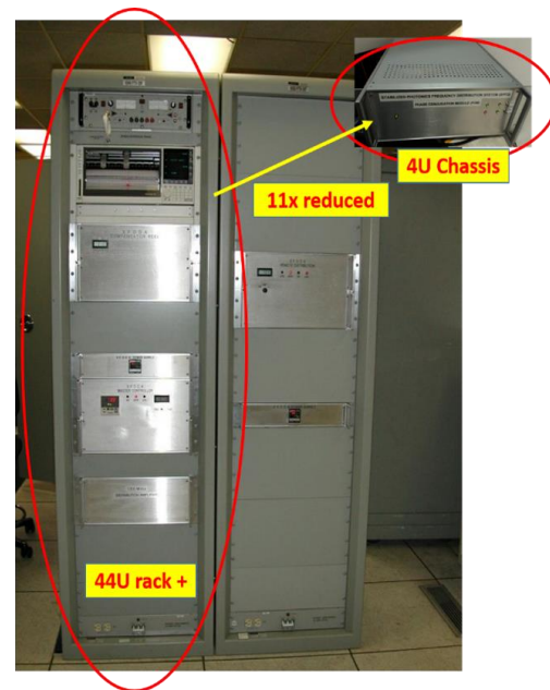
Fig. 1. Phase Conjugation Module (4U chassis) vs SFODA. The size reduced by 11 times
