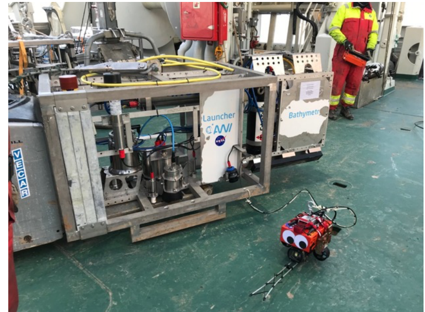
Example of SpongeBob SpareParts next to AWI's OFOBS undersea camera system. The entirety of the highly maneuverable vehicle on the right is about the size of a single high resolution camera on a traditional vehicle.
