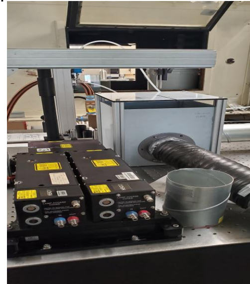
Figure 7: Jet enclosure with hose for particle separator
