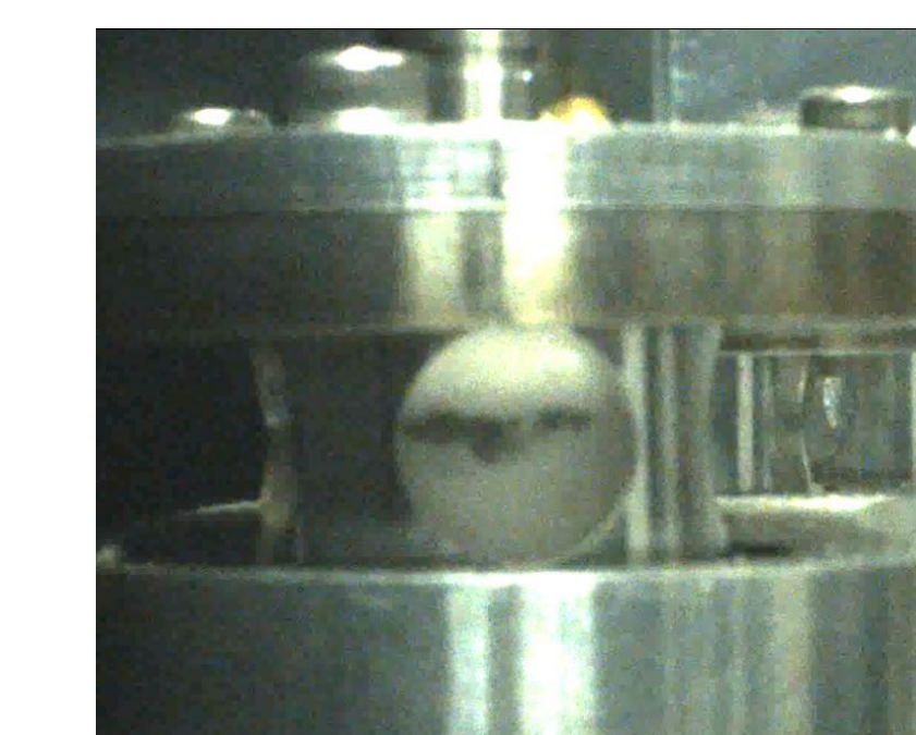
Resulting ice sample filling 5cc science sample chamber
