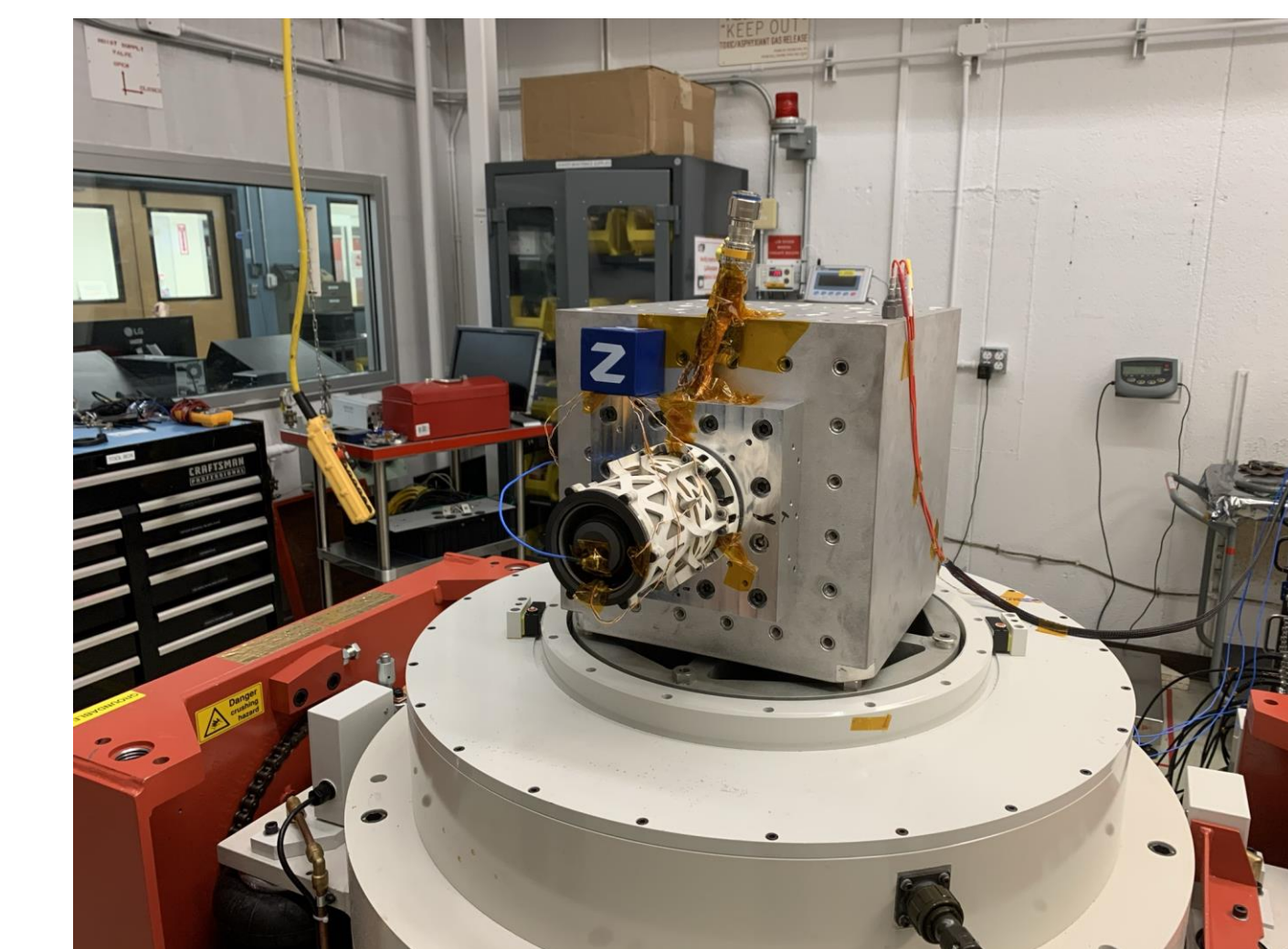
ASTRAEUS thruster at JPL's Environmental Test Lab for dynamic environments testing.
