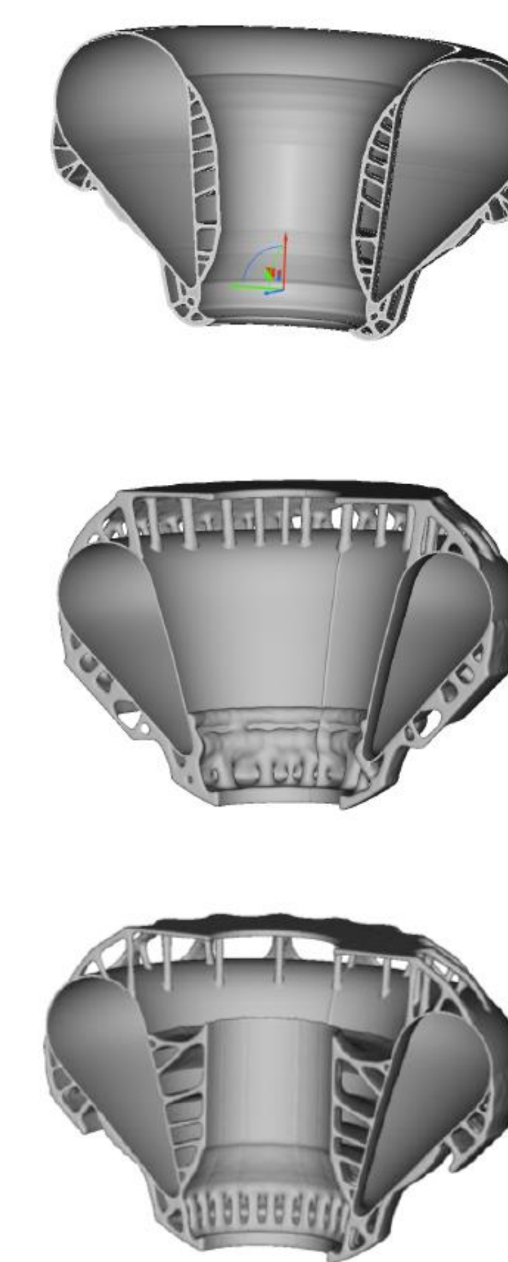
Figure 3: Topological optimization results using axisymmetric (top), 1/4 symmetry (middle) and 1/16th symmetry (bottom). Note the change in complexity in various features.
