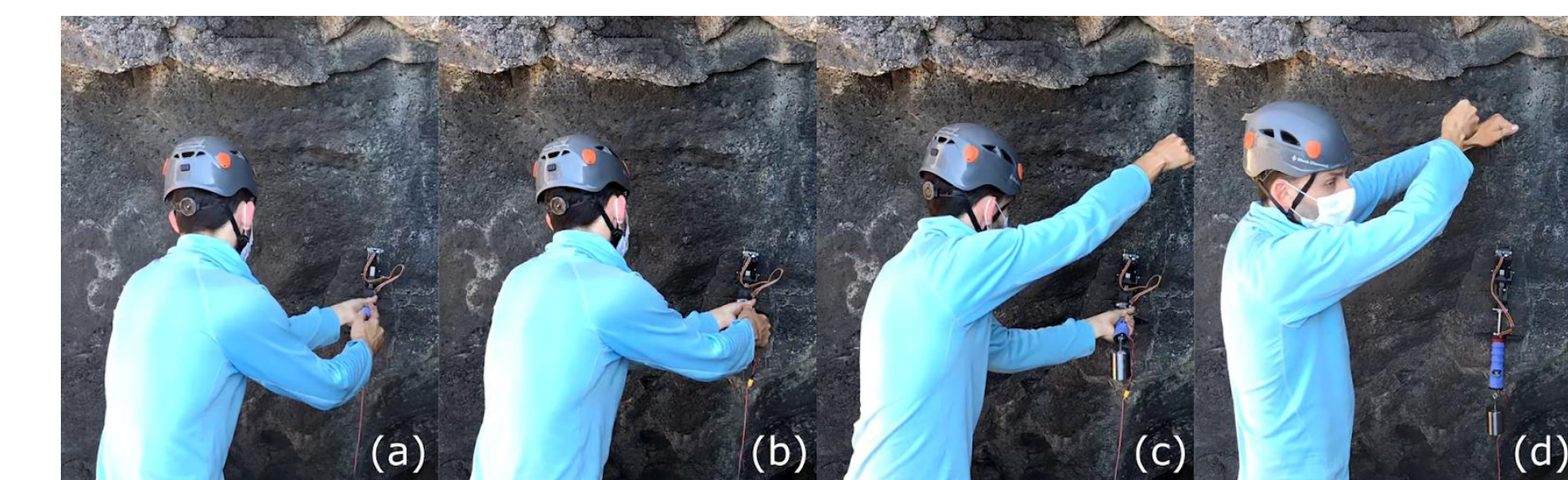
Handheld operation of the gripper at Pisgah, CA: the gripper positioned, gripper engaged (b), the handle rotated downward (c), and handle released (d). The success of the grasp was verified by the gripper supporting 1.5 kg.
