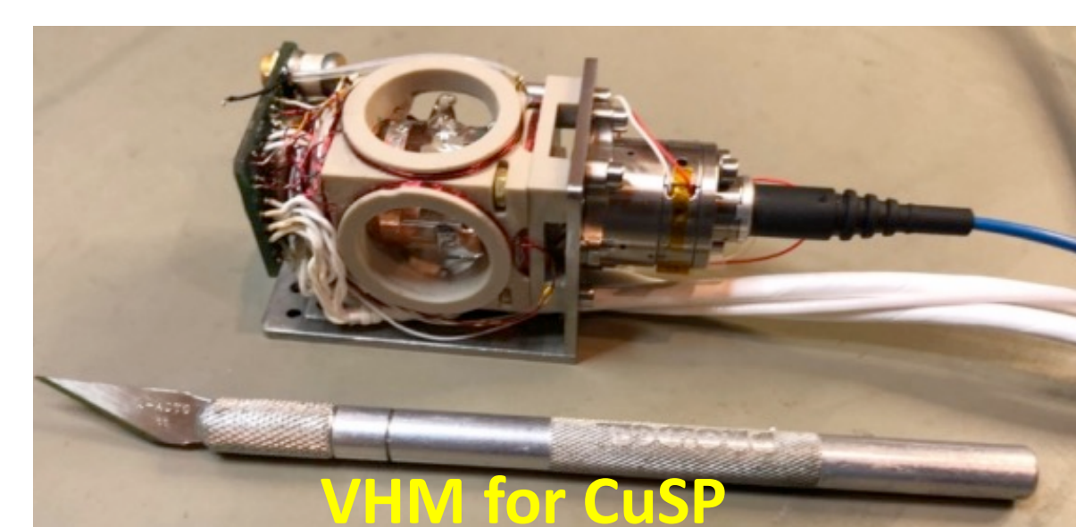
Figure 1. The VHM awaiting launch on the CubeSat for Solar Particles (CuSP) mission is a fourth generation version of the JPL compact laser-pumped helium magnetometer
