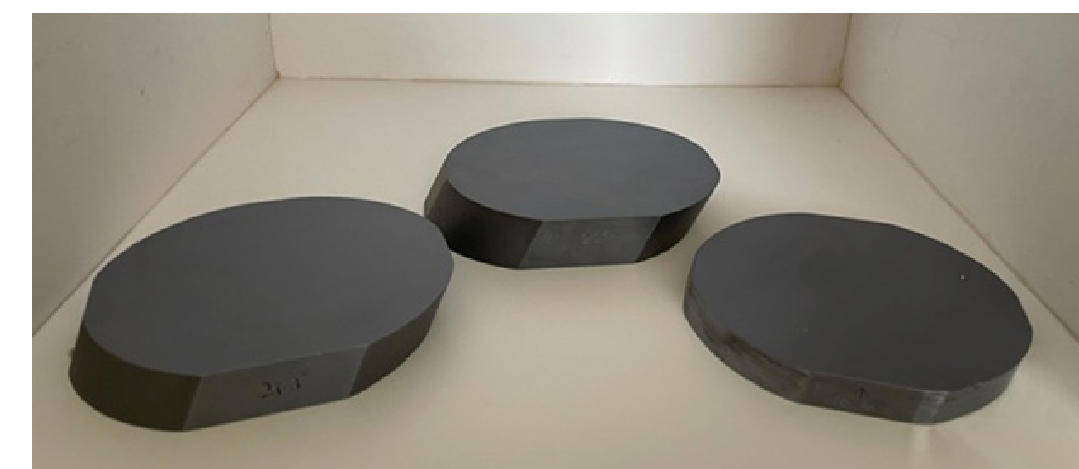
Figure 5. Grating substrates cut from custom crystallographically oriented silicon. Left to right: PARVI echelle, iLocater echelle, iLocater cross-disperser.
