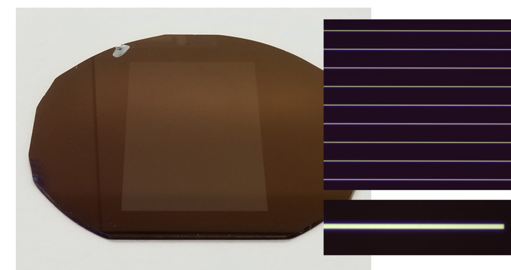
Figure 4. E-beam patterned grating of chromium lines on custom crystallographically oriented silicon wafer (6-inch dia.) to test PARVI grating fabrication process.
