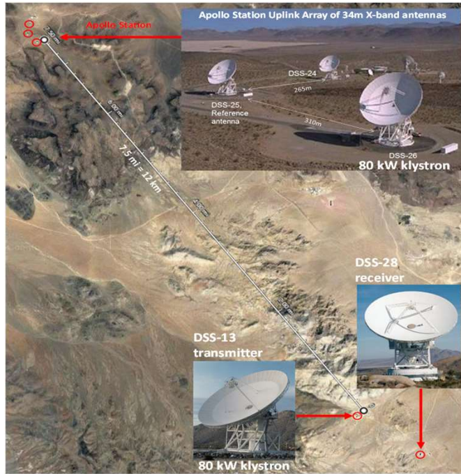
Figure 1. Comparative geography of the short baseline Apollo Array of 3 DSN 34 meter BWG antennas (DSS-24/25/26), and the long baseline 2-element array of DSS-26/13, equipped with 80 kW transmitters.
